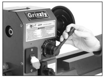
Figure 16. Adjusting spindle speed.
